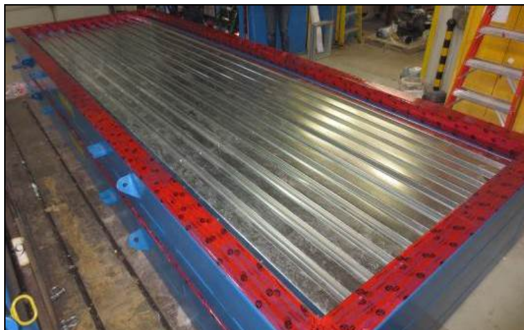
Figure 1 – Roof Test Frame Positioned Steel Deck
