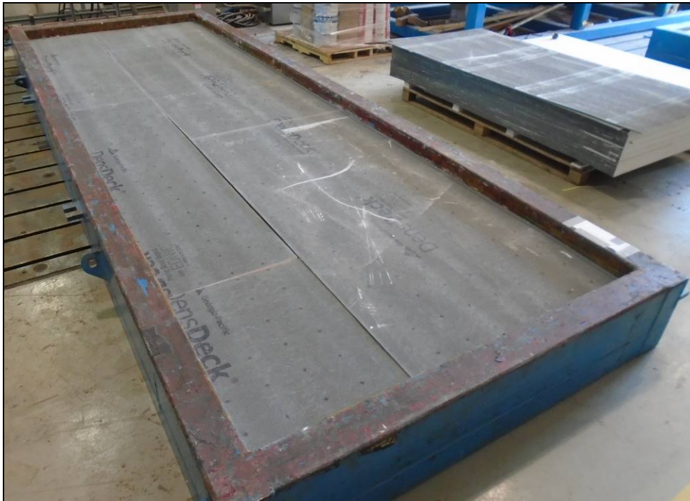
Photo C-2 – DensDeck® Prime thermal barrier ribbon adhered with Parafast Insulation Adhesive C
