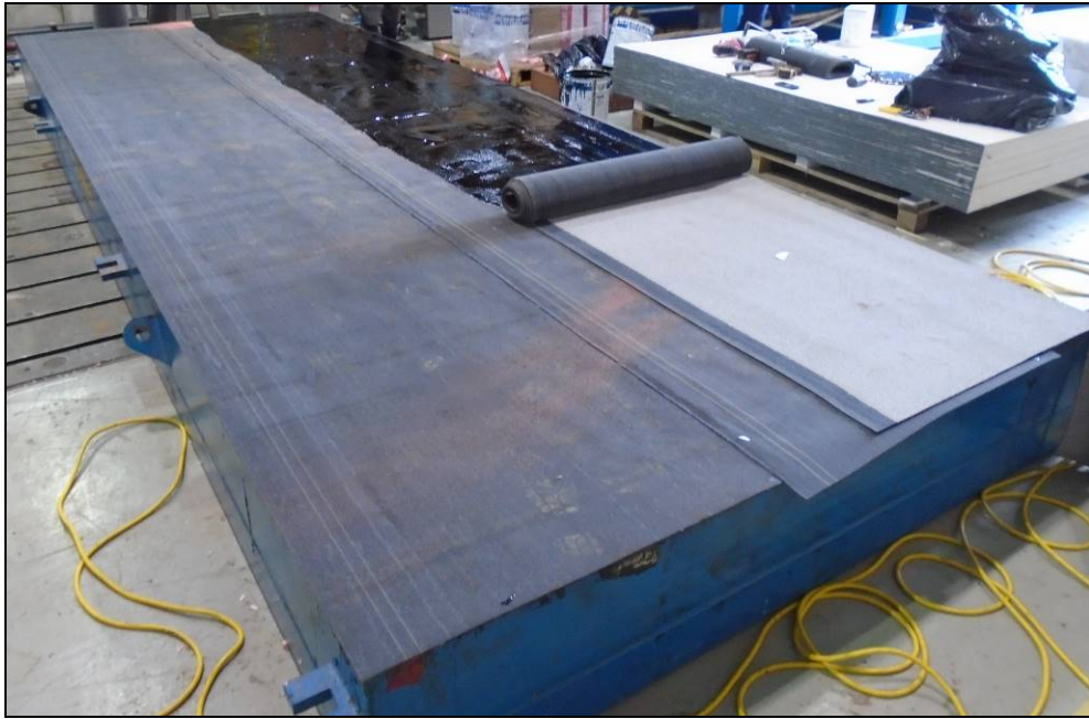
Photo C-9 – Paradiene 30 FR adhered to base sheet with PA-311 R Adhesive
