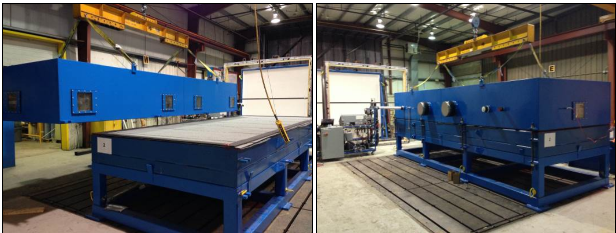
Figure 2 – Stock Photos of Dynamic Wind Uplift Pressure Chamber Connection
