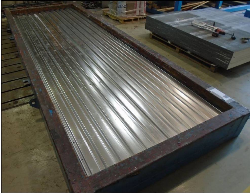
Photo C-1 – Element test frame with steel deck mechanically attached at every flute
