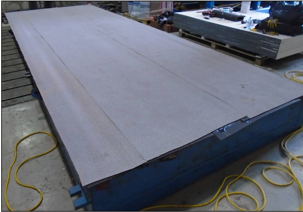
Photo C-11 – Complete AARS specimen in roof test frame
